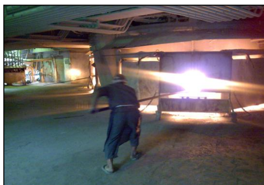
A regular worker working near a furnace without protective gears, BCCL.
