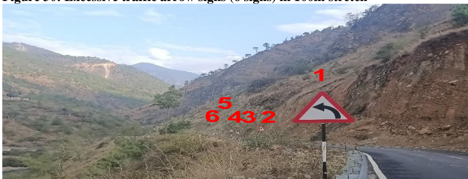
Figure 30: Excessive traffic arrow signs (6 signs) in 100m stretch
