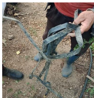
Example case: a drip irrigation set was discarded after it became clogged with mud during its first use and was rendered useless.
