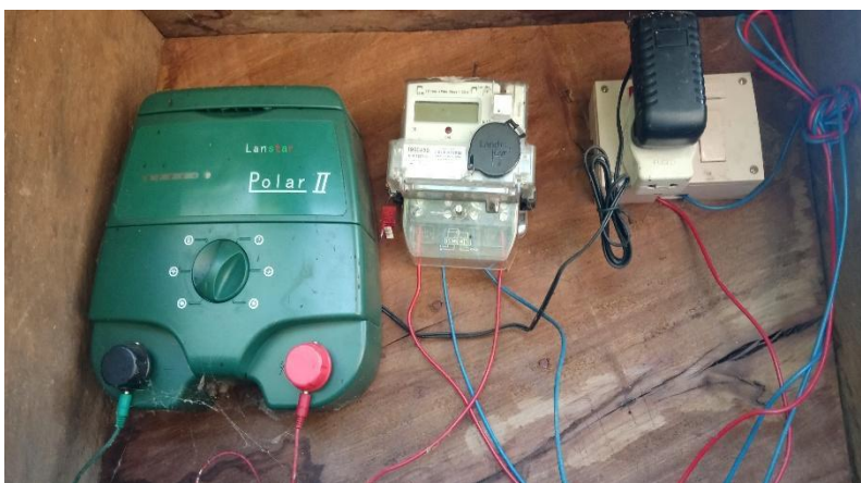
A sample of the energiser used in electric fencing – these devices have been reported to be vulnerable to lightning strikes, requiring farmers to unplug the power supply during storms. However, this is not always feasible, especially when no one is at home during the farming season. If damaged, the energiser must be replaced by purchasing a new one (without subsidies) from a sole supplier based in Thimphu.
